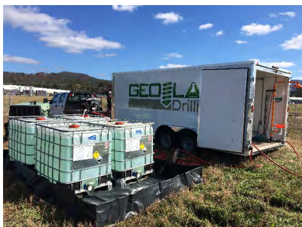
Reagents Stored in Secondary Containment
